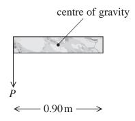
Complete the diagram above by adding labelled arrows to show the positions and directions of the other forces acting on the stone.
